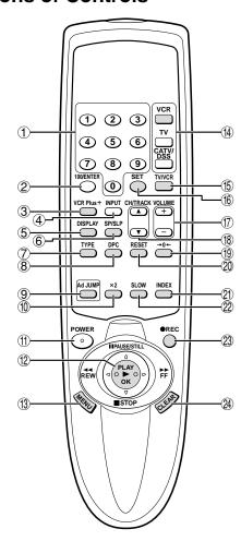
**NOTE:** The shaded buttons are used for VCR operation only.
